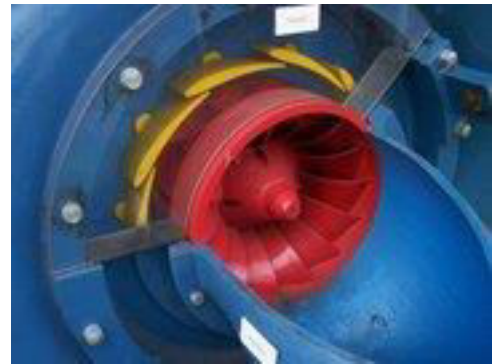
Guide vanes at minimum flow setting
